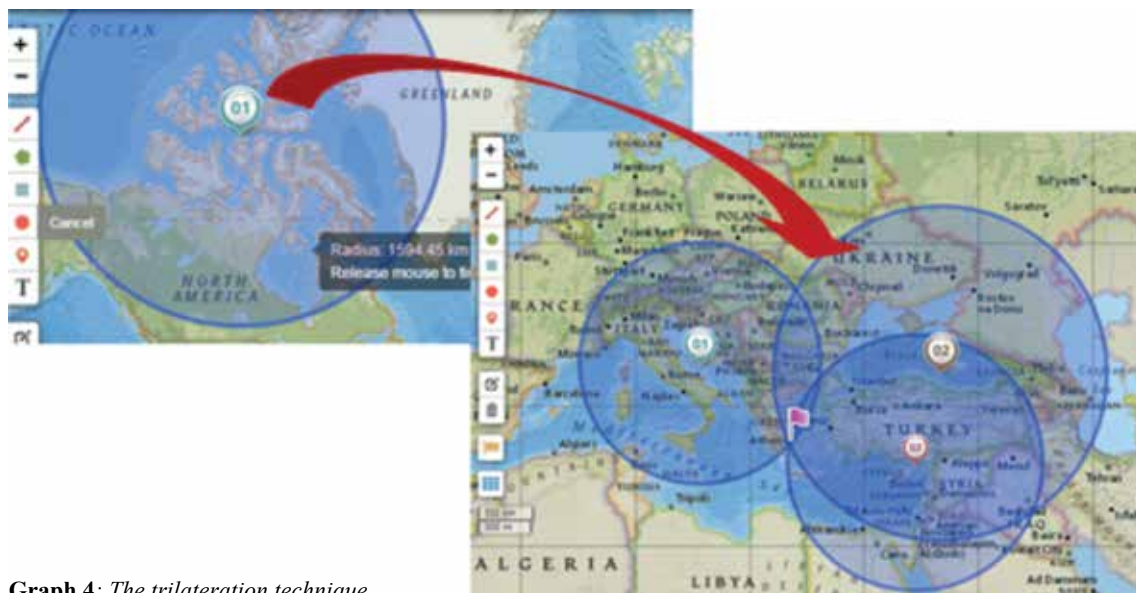
Graph.4: The trilateration technique
