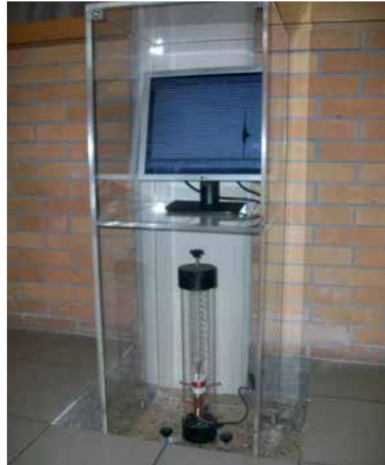
A TC1 seismometer installed in the premises of Ellinogermaniki Agogi in Athens
