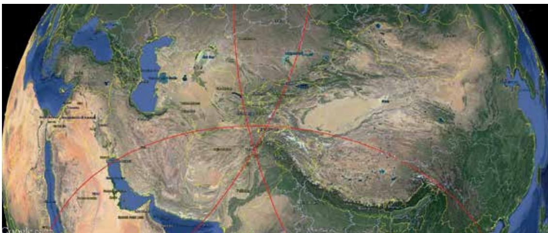
The localization of the epicenter of a teleseism on Google Earth Pro starting from real waveforms
