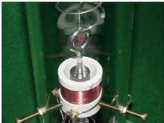
Particular of the magnets oscillating respectively inside the coil (left) and inside the damper (right)
